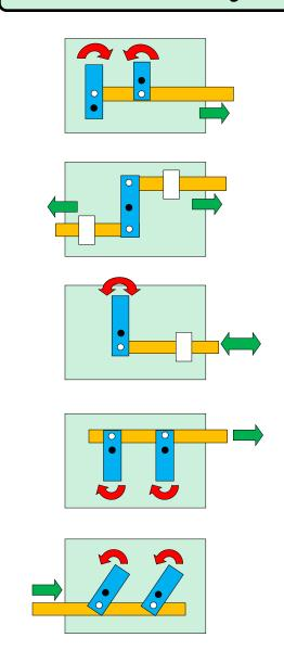
You can create different types of movement by combining different levers and linkages. The way you connect them will change the output movement that is created by the input.
